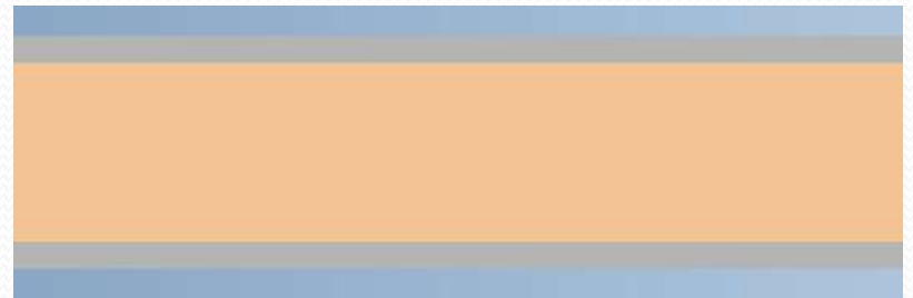
Fiberglass – balsa - Fiberglass
